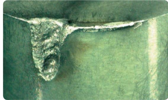
If rough machining is repeated with a constant depth of cut, as shown above, boundary notch wear progresses within a short period of time, making the tool life significantly shorter. The following two machining methods are effective for prolonging the tool life by controlling the boundary notch wear:
