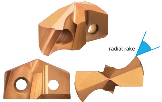
High radial rake enables to restrain wear by reducing heating during cutting.
