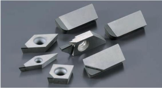
Diamond excels in deposition resistance with its low affinity and has excellent wear resistance with high hardness. But it also has a problem with fracture resistance due to lack of toughness. PCD is the material solving that problem without losing original characteristics of diamond by sintering fine grain diamond and generating polycrystallization. It enables much higher speed machining of nonferrous metals compared to carbide.
