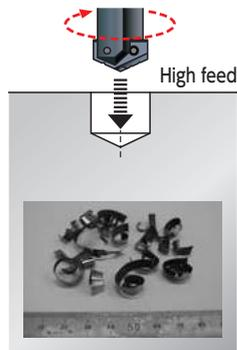
③ Change over to the correct cutting speed and feed rate 1 to 2 mm before reaching the bottom.
