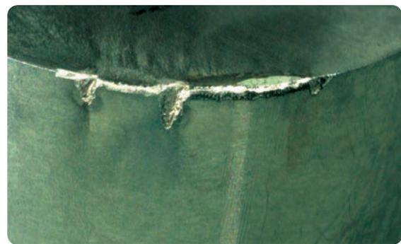
By ramping the insert into cut, the wear is distributed all over the cutting edge as the depth of cut is changed continuously. This method is most suitable for roughing of heat-resistant alloys.
