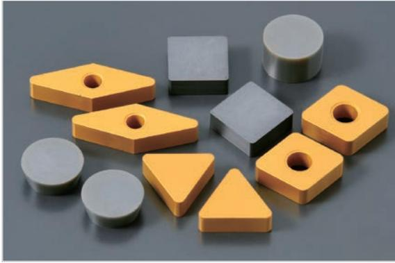
The silicon nitride-based ceramics have approximately twice the fracture toughness of alumina-based, having high fracture resistance equal to some carbide tools. These grades allow for efficient machining in high speed ranges where traditional ceramic tools were not able to perform well, including milling of cast iron and interrupted cutting in poor surface conditions.
