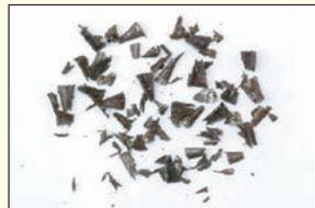
Shape of chips when cast iron was machined.
