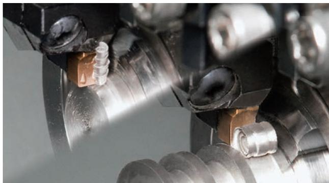
"SCRUM DUO" offers excellent stable machining and longer tool life in grooving and traversing
