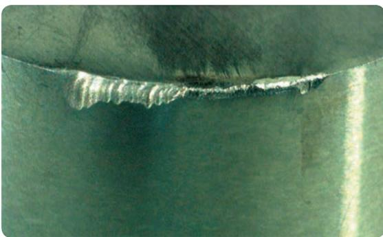
Rough machining with a different depth of cut each pass can cause the boundary notch wear to happen at different contact points, thus the boundary notch wear is spread over a larger area.
