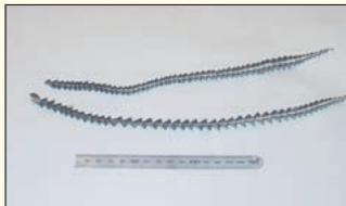
Shape of chips when cut by high-speed tool steel drill
