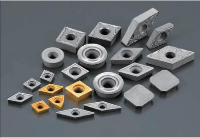
Cermet is a tool material composed mainly of TiC (Titanium Carbide) and TiN (Titanium Nitride). The name, cermet, is derived from the words CERAMIC and METAL (representing carbide). As the name suggests, cutting performance is also in the mid-range of ceramic's and carbide's. The advantages of this material grade are that high-quality and excellent surface finishes can be achieved allied with elevated cutting speeds
