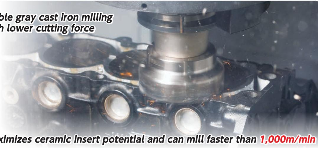
● **Maximizes ceramic insert potential and can mill faster than 1,000m/min**
